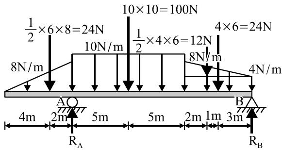
$$(1) \sum M_A = 0 \\ 10 \times 10 \times 5 + \frac{1}{2} \times 4 \times 6 \times 12 + 4 \times 6 \times 13 - \frac{1}{2} \times 6 \times 8 \times 2 - R_B \times 16 = 0 \\ \therefore R_B = 56.75 \text{ N} (\uparrow)$$
