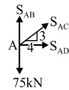
$$\sum F_y = 0 \quad \frac{3}{5} S_{AC} + S_{AB} - 75 = 0 \\ \therefore \frac{3}{5} S_{AC} + 48.6 - 75 = 0 \quad \therefore S_{AC} = 44 \text{ kN} (\text{T})$$
